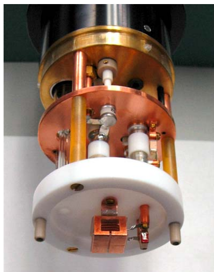
Fig. 1. 900 MHz 1 H-X, 500 µL flat coil probe for oriented membrane proteins.
