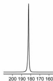
Fig. 7 Quantification of the polarization achieved with PASADENA. ^{13}\text{C} hyperpolarized spectrum of 2.7 mmol/L HEP 1\text{-}^{13}\text{C} , 2,3,3\text{-d}_3 at 4.7 T in vitro (a). Polarization of \sim 18\% was achieved in this representative example. The inset spectrum shows a reference signal obtained from natural abundance ethanol; ^{13}\text{C} concentration = 188 mmol/L per site (b). Note that the scale of the inset spectrum was magnified by 512 times
